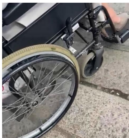
The wheelchair's small front wheels can easily get stuck in gaps between paving slabs.
